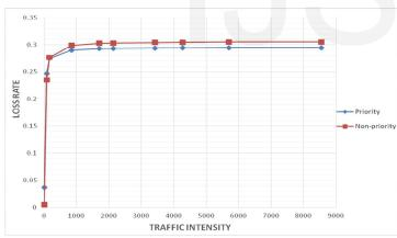
Fig. 4.4: Loss rate as a function of traffic intensity
